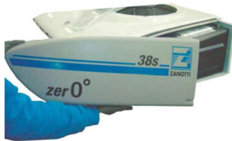
Figure 13 - Removing the side frame
