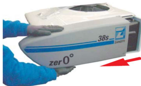
Figure 12 - Sliding the side frame
