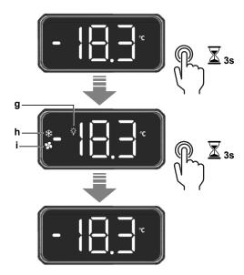
This screen shows activated functions and outputs icons overlapped with temperature value.
