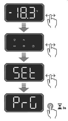
3 Navigate through the programming screen menu by swiping horizontally through the screens.
