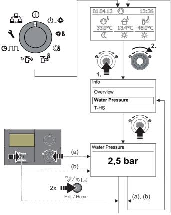
Fig. 3-6 Displaying info values (e.g. system pressure)
