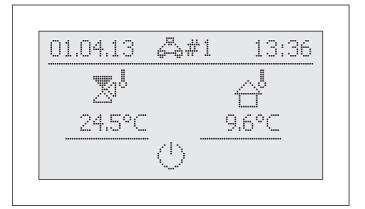
Fig. 3-11 Example of the display for the remote-controlled mixer module
