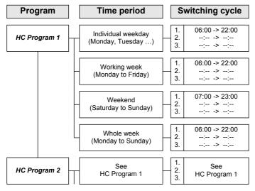
Tab. 3-8 Menu structure of heating circuit/time program
