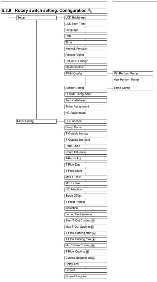
Tab. 5-12 M Parameters in the "Configuration" rotary switch setting
