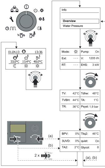
Fig. 3-5 Displaying the operating data overview
