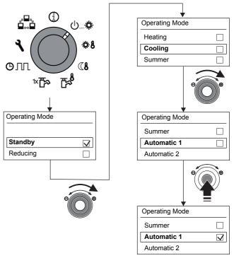
Fig. 3-7 Changing the operating mode (e.g. from "Standby" to "Automatic 1")
