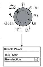
Fig. 3-9 Display of the "Remote Param" level during commissioning or after interim disconnection from the mains
