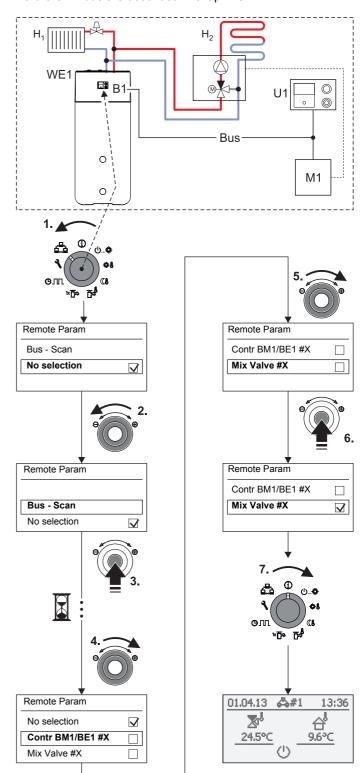
RoCon B1 control panel of the Altherma M ECH2O R1 Bus CAN bus (connection line between RoCon devices
