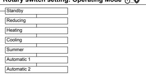
Tab. 5-4 Parameters in the "Operating Mode" rotary switch setting
