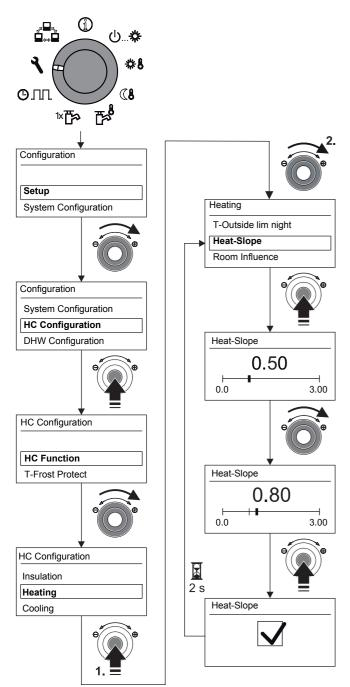
Fig. 3-14 Manual setting of the heat slope (illustration with "User" access authorisation)
