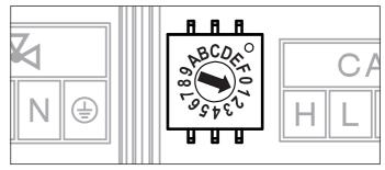
Fig. 4-2 Setting the device ID for the EHS157068 mixer module
