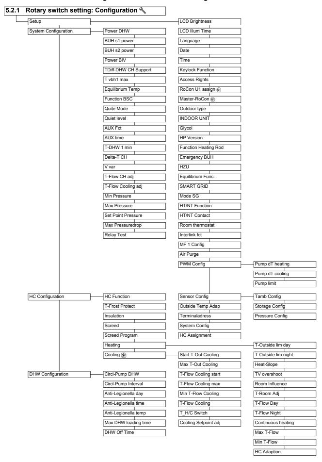
Tab. 5-2 Parameters in the "Configuration" rotary switch setting
