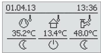
Fig. 3-8 Standard display in the "Standby" operating mode (above the frost limit temperature)
