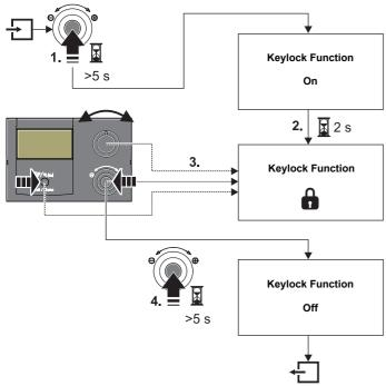
Fig. 3-4 Activating (1.) and deactivating (4.) the key lock
