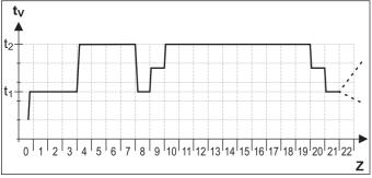
Fig. 3-19 Chronological sequence of the screed program during the combined function and screed curing heating (for legend, see fig. 3-18)
