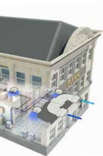
You can use the decorative elements on a building's façade, such as pediments or logos, to hide the grilles making the installation completely invisible
