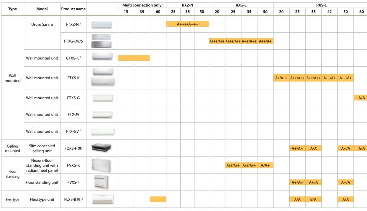
Note: (1) These indoor units can only be used in pair application (2) These indoor units can only be used in multi application. For FLXS-B, remark is only valid for 60-class.
